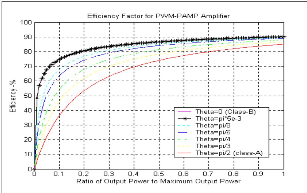
Fig. 12: Predicted Efficiency of PWM-PAMP. Theta = 0 and Theta = pi\*5e-3 overlay each other.
