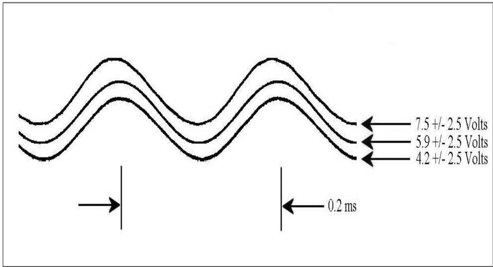
Fig. 22: 5 kHz Sinusoid Output and Tracking Rails
