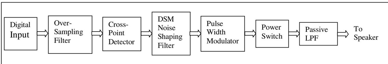
Fig. 6: PWM DAC/Class-D Amplifier
