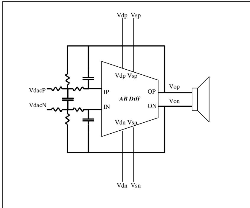
Fig. 11: Smoothing Filter and Power Amplifier
