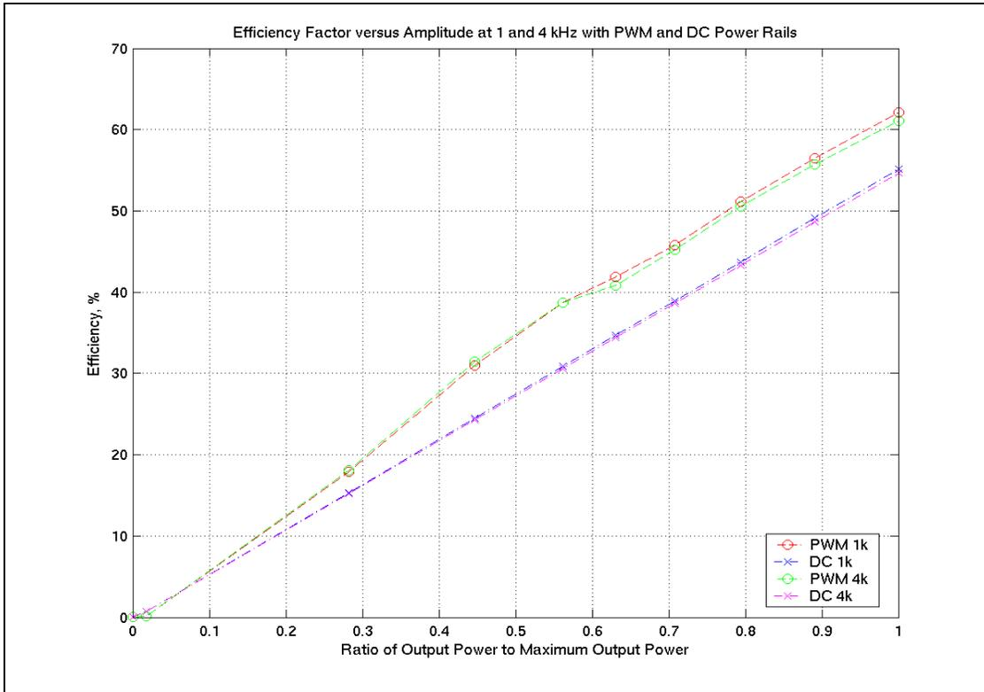
Fig. 16: Efficiency Comparison. 1 and 4k PWM traces overlay. 1 and 4k DC traces overlay.
