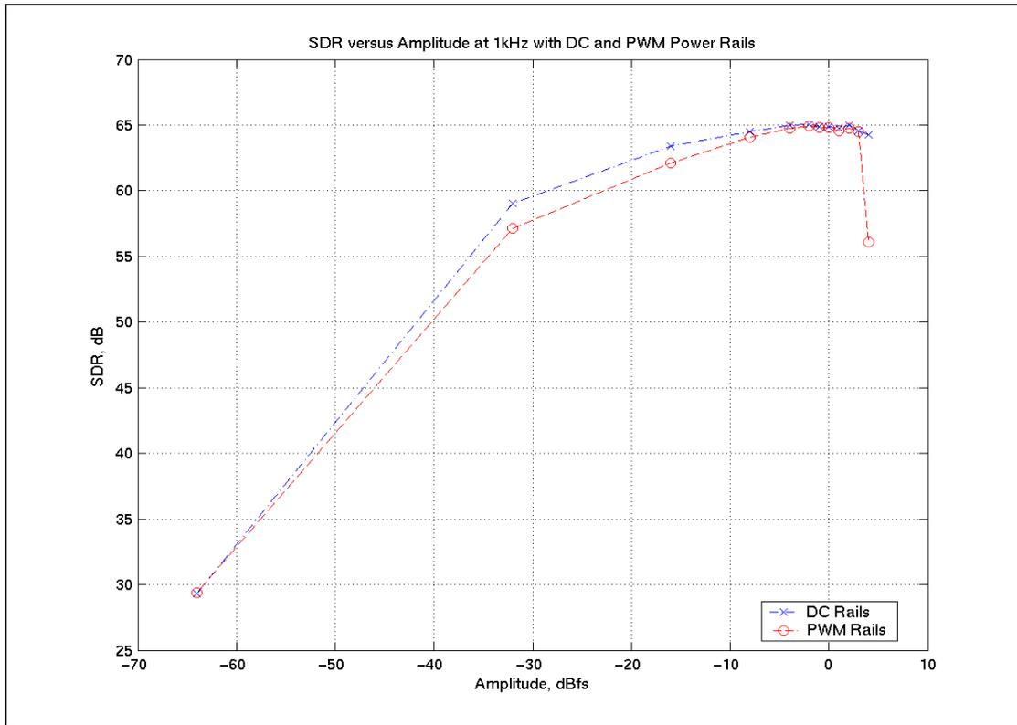
Fig. 15: SDR versus Amplitude at 1 kHz for DC and PWM
