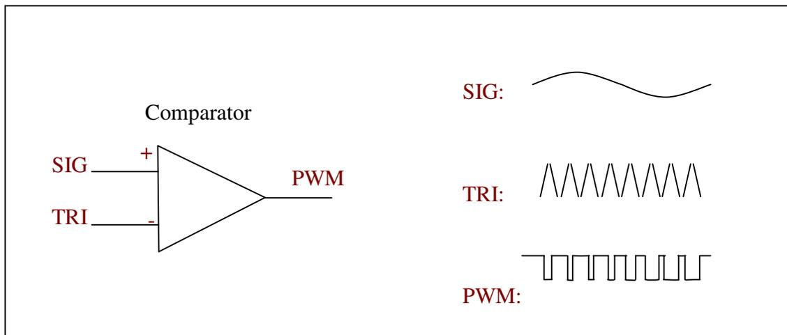
Fig. 5: Comparator and Waveforms for Analog Class-D
