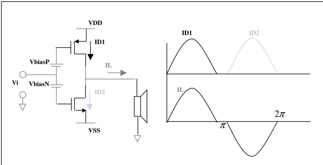
Fig. 2: Class-B Output Stage and Current Waveforms
