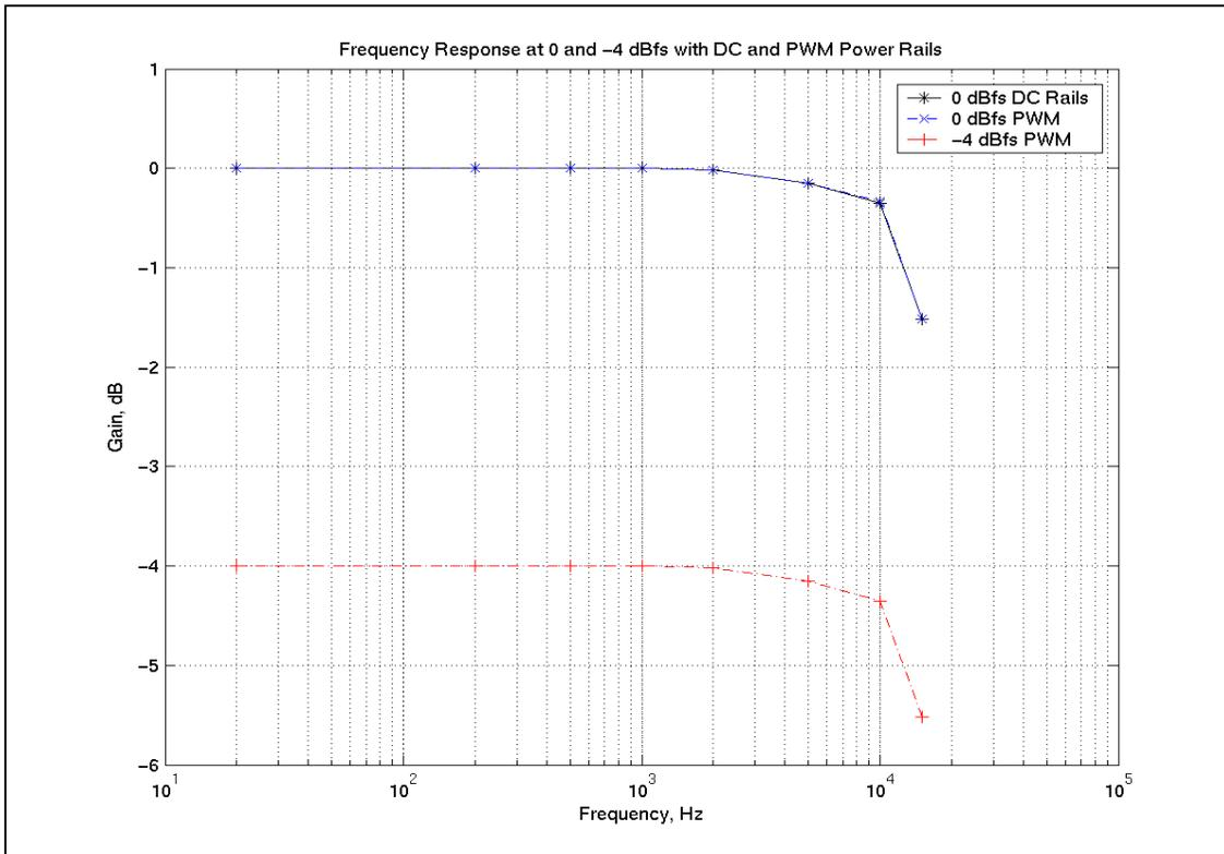
Fig. 17: Frequency Response. PWM and DC 0 dB traces overlay each other.
