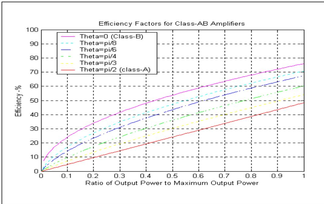
Fig. 13: Predicted Efficiency of Class-AB Amplifier
