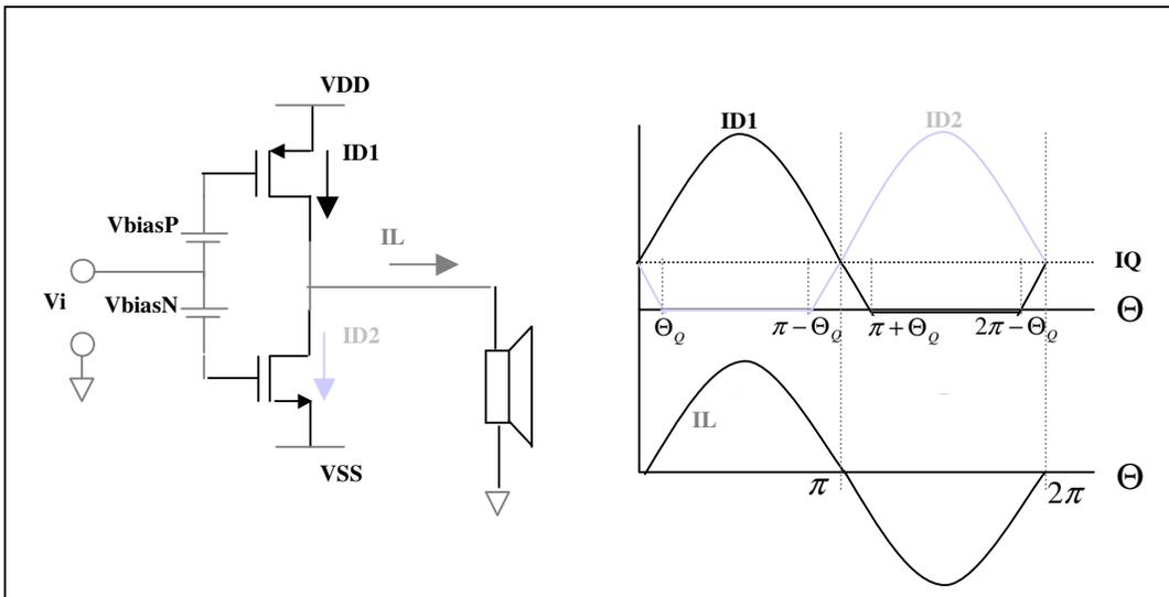
Fig. 3: Class-AB Output Stage and Current Waveforms
