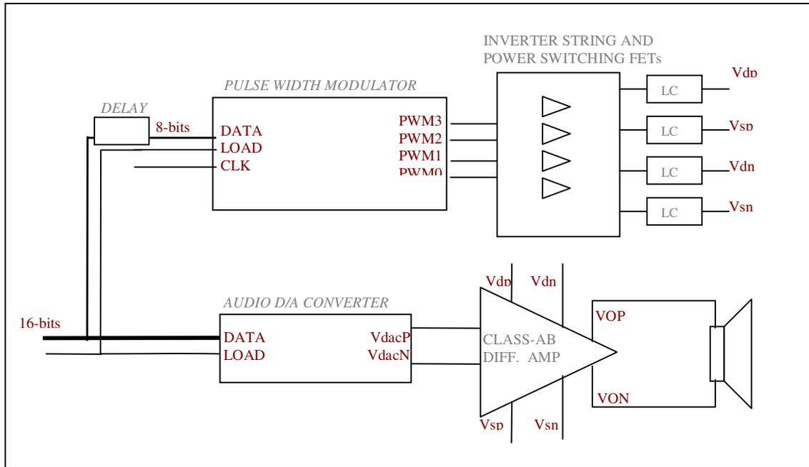
Fig. 7: Top Level Block Diagram of PWM-PAM
