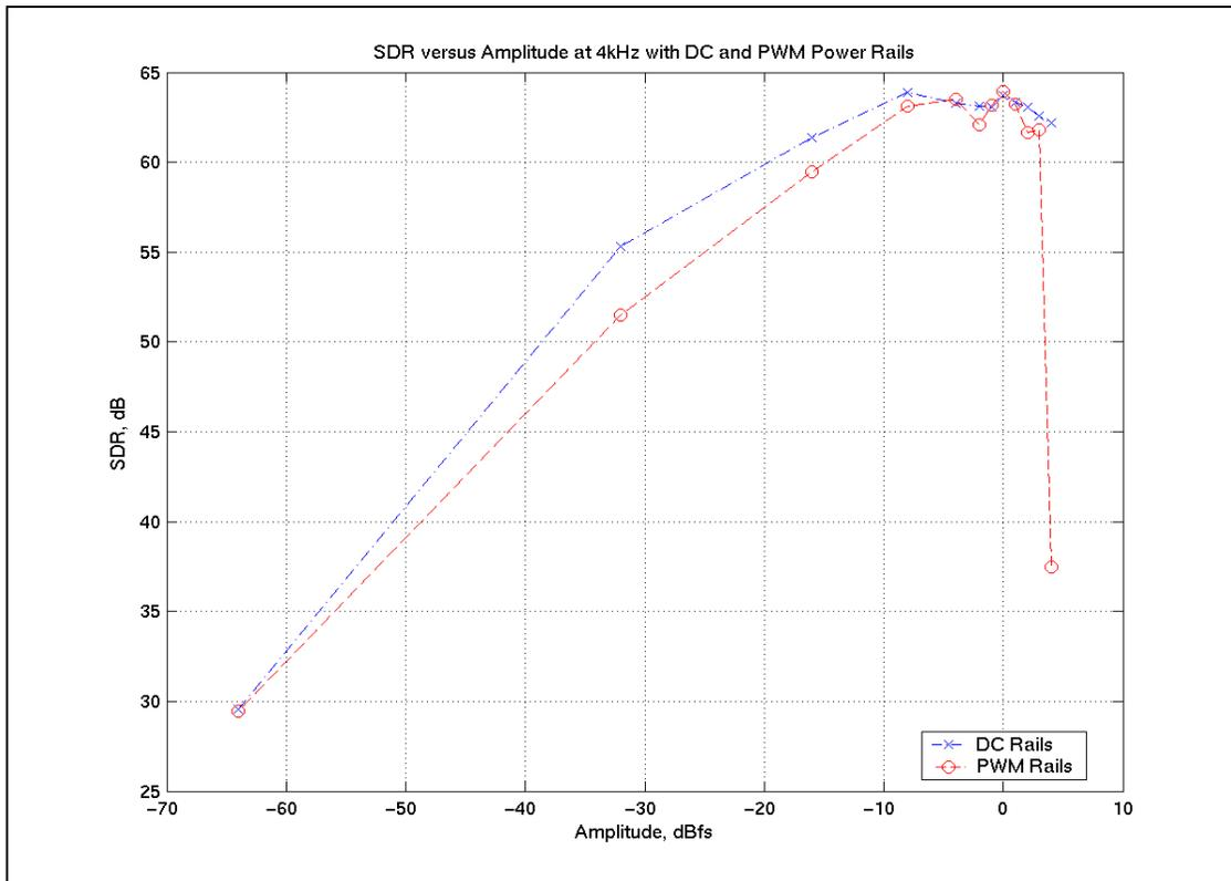
Fig. 14: SDR versus Amplitude at 4 kHz for DC and PWM
