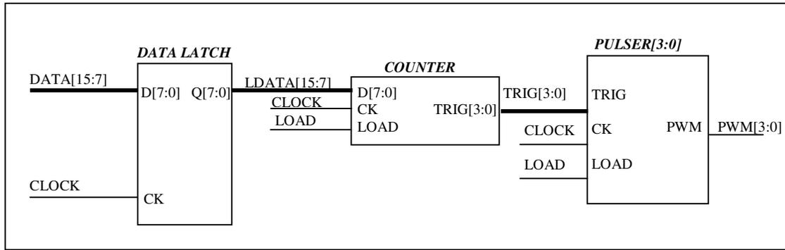
Fig. 10: Pulse Width Modulator Block Diagram
