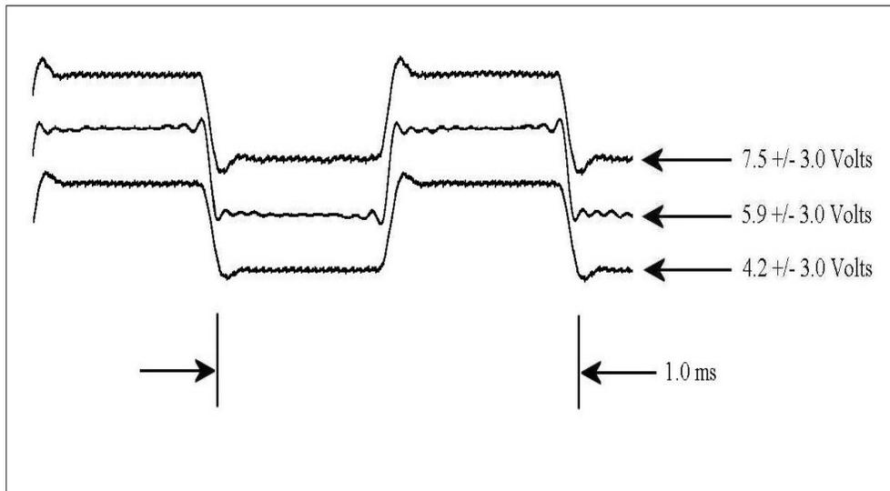
Fig. 23: 1 kHz Square Wave Output and Tracking Rails
