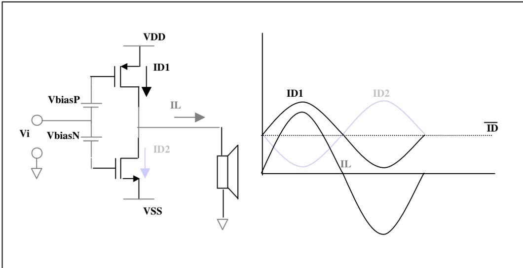
Fig. 1: Class-A Output Stage and Current Waveforms
