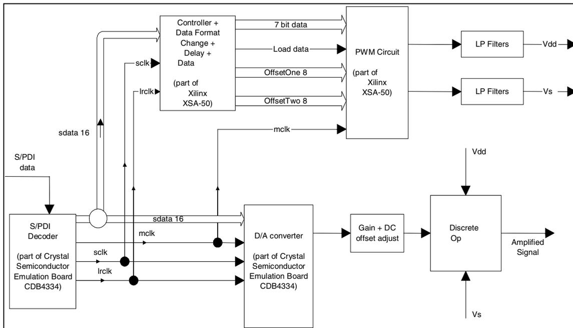
Fig. 19: Block Diagram of Hardware Prototype
