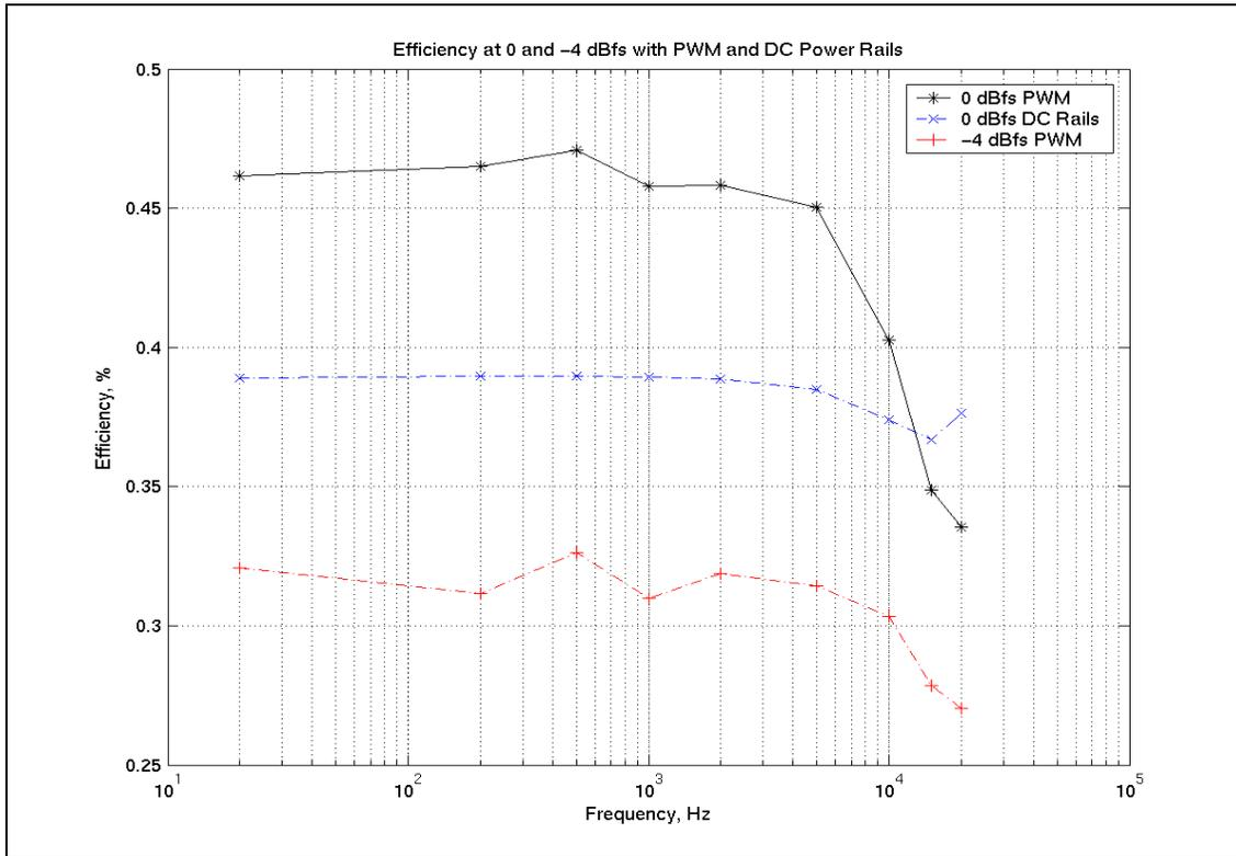
Fig. 18: Efficiency versus Frequency
