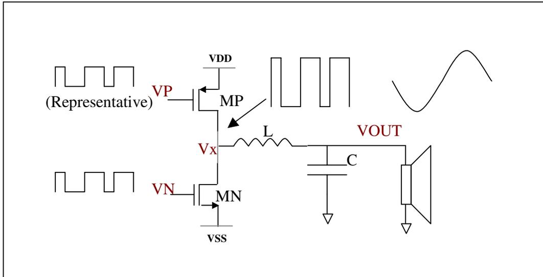
Fig. 4: Class-D Output Stage and Voltage Waveforms
