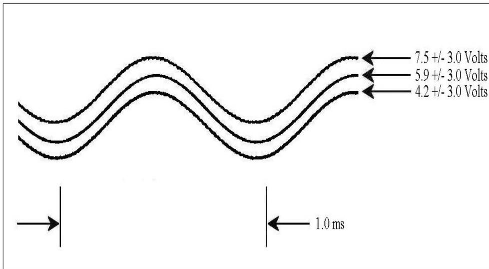
Fig. 21: One kHz Output and Tracking Rails
