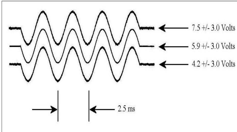
Fig. 20: 400 Hz Burst Output and Tracking Rails
